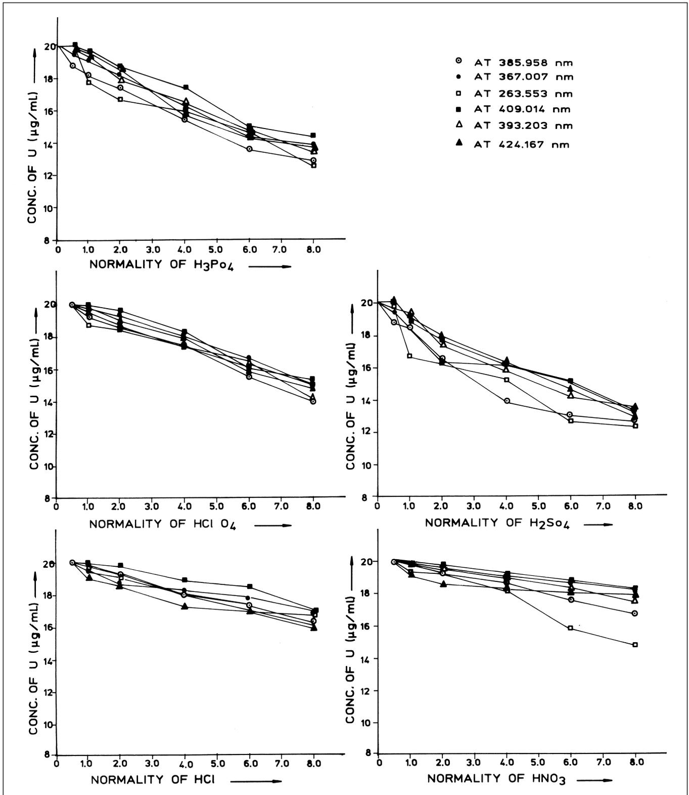
Fig. 1. Effect of different acids on uranium (20 µg/mL).
