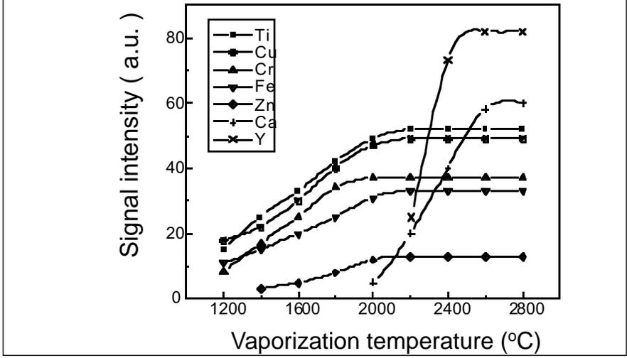
*Fig. 3. Analytical signal versus vaporization temperature with PTFE: Ti, 0.2  $\mu\text{g mL}^{-1}$ ; Cu and Fe, 0.6  $\mu\text{g mL}^{-1}$ ; Cr, 0.4  $\mu\text{g mL}^{-1}$ ; Zn, 10  $\mu\text{g mL}^{-1}$ ; Ca, 0.1  $\mu\text{g mL}^{-1}$ ; Y, 1.5  $\mu\text{g mL}^{-1}$ .*
