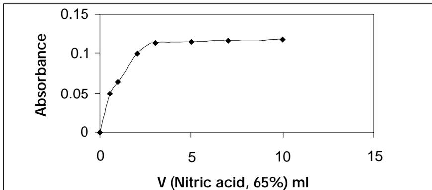
*Fig. 1. Acidity dependence of the Cr(VI)-TBAB ion-pair stability: [TBAB]=0.02 M, shaking time=5 min and [Cr(VI)] = 1 µg/L.*
