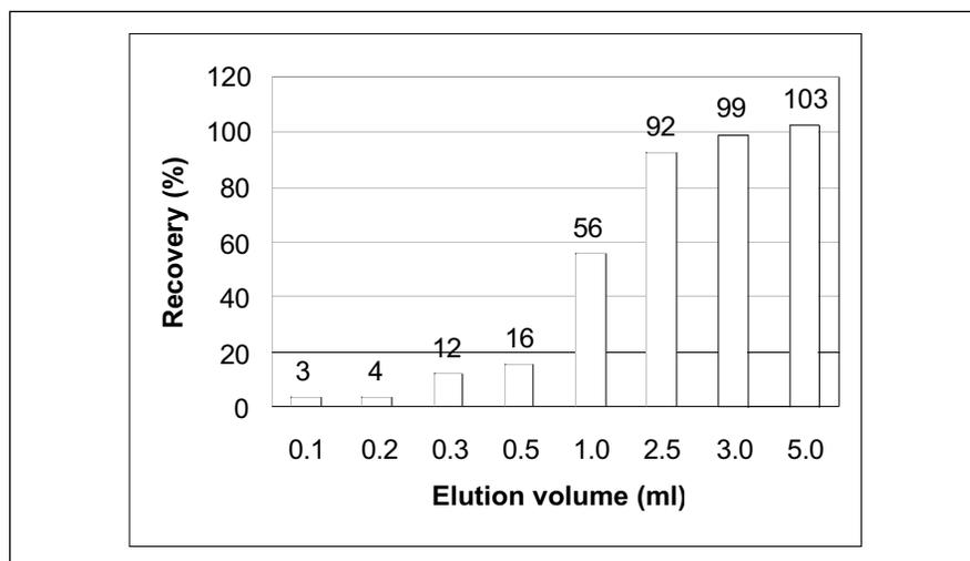
Fig. 3. Minimum elution volume of HCl necessary to strip As(V) quantitatively from the column. Figures in the top of the bars indicate the percentage of As(V) recovery.
