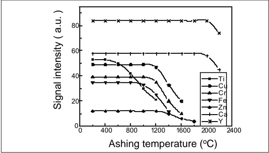
*Fig. 2. Influences of ashing temperature on signal intensity with PTFE: Ti, 0.2  $\mu\text{g mL}^{-1}$ ; Cu and Fe, 0.6  $\mu\text{g mL}^{-1}$ ; Cr, 0.4  $\mu\text{g mL}^{-1}$ ; Zn, 10  $\mu\text{g mL}^{-1}$ ; Ca, 0.1  $\mu\text{g mL}^{-1}$ ; Y, 1.5  $\mu\text{g mL}^{-1}$ .*
