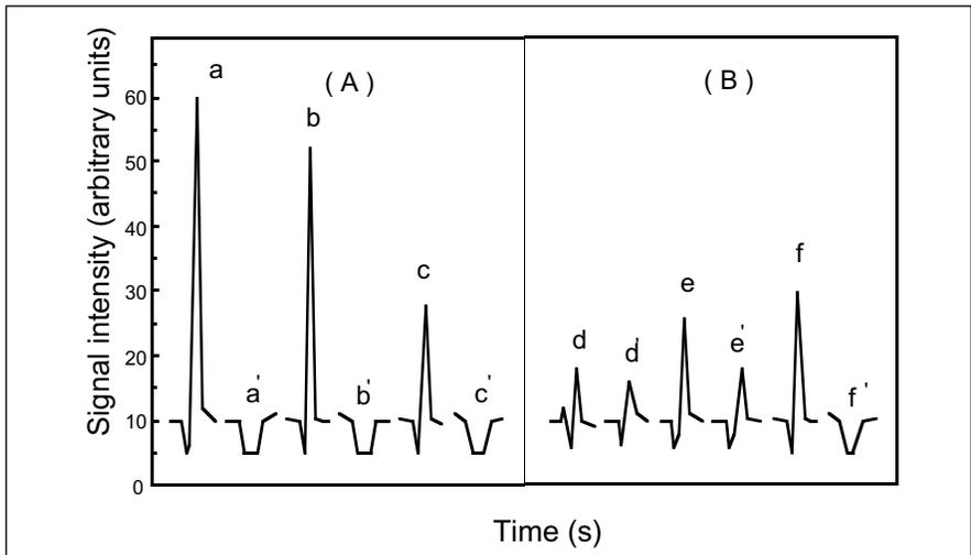
*Fig. 1. Comparison of analytical signals for Ti, Cu, and Zn. (A) with PTFE: a = 0.2  $\mu\text{g mL}^{-1}$  Ti; b = 0.6  $\mu\text{g mL}^{-1}$  Cu; c = 20  $\mu\text{g mL}^{-1}$  Zn. (B) without PTFE: d = 10  $\mu\text{g mL}^{-1}$  Ti; e = 3.0  $\mu\text{g mL}^{-1}$  Cu; f = 20  $\mu\text{g mL}^{-1}$  Zn; a', b', c', d', e', and f' are their residual signals of the empty firing, respectively.*
