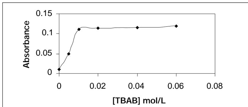
Fig. 2. TBAB concentration effect on the ion-pair extraction: Volume of nitric acid (65%) = 5 mL, shaking time = 5 min and [Cr(VI)] = 1 µg/L.
