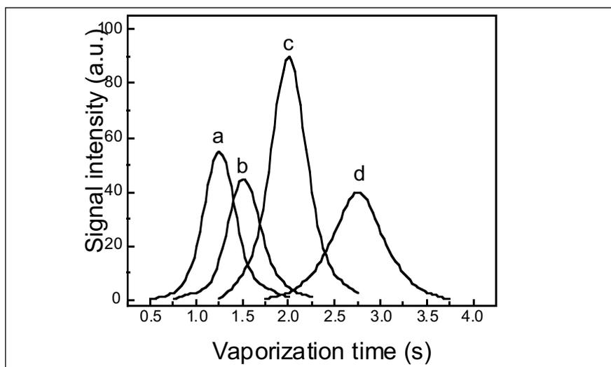
*Fig. 4. Analytical signals vs. vaporization time in the presence of PTFE. A = Zn, 5.0 mg mL<sup>-1</sup>; b = Na, 5.0 mg mL<sup>-1</sup>; c = Y, 1.0 µg mL<sup>-1</sup>; d = Ca, 5.0 mg mL<sup>-1</sup> using 2400°C.*
